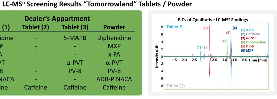
Semi-Quantitative LC-MS<sup>n</sup> Screening ADB-PINACA MS<sup>1</sup> data of the [M+H]<sup>+</sup> ions of ADB-PINACA (m/z 345.2) and D9-ADB-PINACA was used for semiquantitative evaluation of the screening results.
