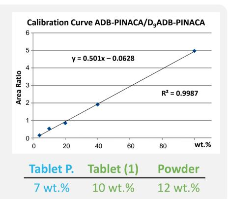
were used for compound identification. Additionally, a semi-quantitative evaluation of the screening data was used to estimate the ADB-PINACA content of the tablets. A 5-point calibration using D9-ADB-PINACA as internal standard in LC eluent was prepared.
