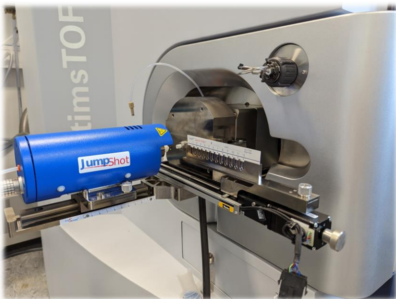
Fig. 2: Bruker timsTOF Pro 2 equipped with a Bruker DART JumpShot ion source.
